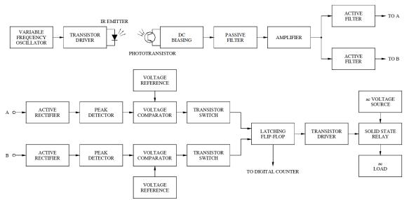
FIG 8. IR detector and emitter block diagram of the analog circuitry<sup>3</sup>
