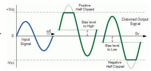
**FIG 2.** Non-linear amplitude distortion due to incorrect biasing<sup>1</sup>
